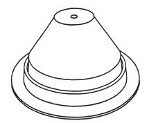
4" high, 7-3/4" base diameter, for use with assemblies using No. 684T or No. 684CT tubular pitch pans.
