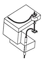
Cat. No. 743CDCT — Copper Clamp to Copper Tee Connector - 3 lbs. - 5 oz. Cat. No. 743ADCT — Aluminum Clamp to Copper Tee Connector - 3 lbs. - 1 oz. Cat. No. 743ADAT — Aluminum Clamp to Aluminum Tee Connector - 2 lbs. - 11 oz.
