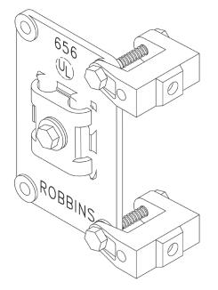
Heavy cast bronze or aluminum metal bonding plate – over 8 square inches of contact surface and 1-1/2" cable contact. Cap may be rotated for alternate cable position. Provided with 2 cast, "C" clamps to fasten to steel surface. For main sized cables through No. 605. Overall dimensions - 2-1/4" x 4".
