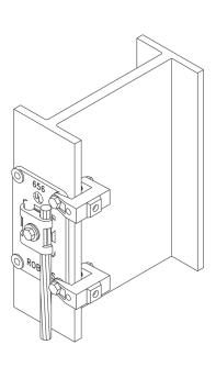
Typical use on steel column showing both cap positions.
