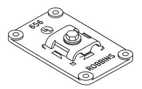
Heavy cast bronze or aluminum metal bonding plate — over 8 square inches of contact surface and 1-1/2" cable contact. Cap may be rotated for alternate cable position. May be fastened to metal surface with bolts and nuts or may be brazed. For main sized cables through No. 605. Overall dimensions -  $2-1/4" \times 4"$ .
