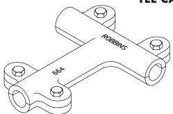
with two 1/4" bolts for tension on cable -1-3/4" cable contact each direction - for main sized cables through No. 605. Overall dimensions  $-1-3/4" \times 2-3/8"$ .
