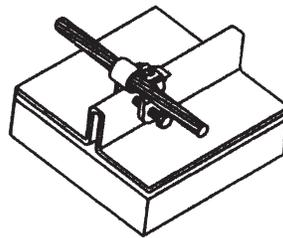
Machined brass or aluminum hexagonal holder for use on standing seams, steel beams, etc. where no penetration of metal is desired or permitted. Comes with No. 72 or No. A72 loop, which can be attached to 1/4" stainless bolt, 1/4" stainless nut for tightening loop. Rubber cap included on bolts to prevent damage to roof. For main and secondary cables and wires.
