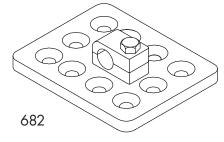
Adhesive cable holder of heavy cast bronze or aluminum. Should be placed on flat or gently sloping roof surface in a bed of hot pitch or approved adhesive. For main sized cables through 604. Overall dimensions - 2-3/4" x 2-1/4''. Adhesive contact area - 6.19 in<sup>2</sup>.
